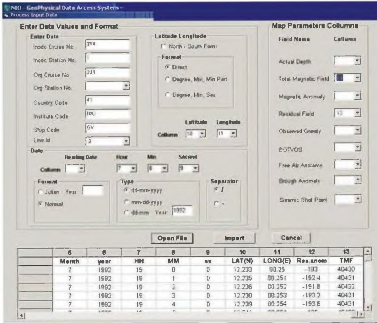
Figure 1. Import module screen of GPDAMS. Data file to be formatted is viewed in lower window screen and administrator requires filling-in of IODC cruise and fix number, and other header information before importing in main database.
