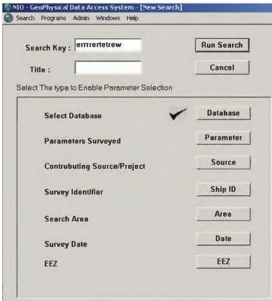
Figure 3. Search screen allows user to select various options like area selection, parameter surveyed, vessel and survey identifier, from date and to date, within or outside EEZ, etc. and help in building the query for retrieving desired data.
