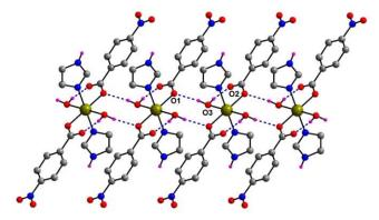
**Figure 2.** Formation of a H-bonded chain along *a* axis via  $O-H\cdots O$  interaction showing the linking of coordinated water (O3) with a coordinated 4-nitrobenzoate of a neighbouring molecule (O1). H atoms attached to C are not shown for clarity.
