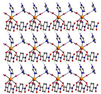
**Figure 6.** Cross-linking of H-bonded chains of hexacoordinated Ca(II) complexes by free as well as coordinated imidazole through N–H···O interactions. H atoms attached to C are not shown for clarity.
