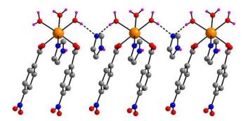
**Figure 5.** Linking of hexacoordinated Ca(II) complexes by the free Im with the aid of  $O-H\cdots N$  interactions leading to the formation of a H-bonded chain along the *b* axis. H atoms attached to C are not shown for clarity.
