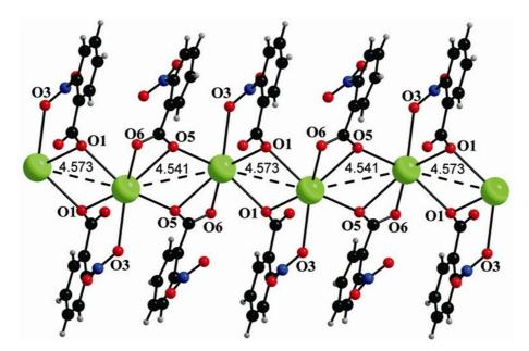
**Figure 4.** A view along *a* showing the 1-D polymeric chain of 1. Alternating pairs of Ba(II) ions are linked by a pair of tridentate ( $\mu_2$ -2-nba-O,O,O-NO<sub>2</sub>) and ( $\mu_2$ -2-nba-O,O,O') ligands resulting in alternating Ba···Ba distances of 4.5406(15) and 4.5726(14) Å. For clarity, the coordinated water molecules on Ba(II) are not shown.
