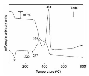
**Figure 1.** TG-DSC thermogram of  $[[Ba(H_2O)_3]_2(\mu_2-2-nba-O,O,O-NO_2)_2(\mu_2-2-nba-O,O,O')_2]_n$  **1.** (Heating rate 10 K/min; Air atmosphere).
