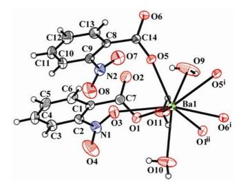
**Figure 2.** The coordination sphere of Ba(II) in  $[[Ba(H_2O)_3]_2(\mu_2-2-nba-O,O,O-NO_2)_2(\mu_2-2-nba-O,O,O')_2]_n$ **1** showing the atom-labelling scheme. Displacement ellipsoids are drawn at the 50% probability level except for the H atoms, which are shown as circles of arbitrary radius. Symmetry code: (i) [-x + 1, -y + 1, -z + 1]; (ii) [-x + 1, -y + 2, -z + 1].
