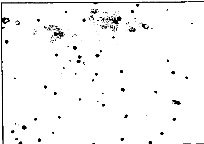
Photomicrograph of ^{239}\text{Pu} alpha particle in PADC film Magnification : 80 X. Exposure : 703703 dpm ^{239}\text{Pu} source at 2.0 cm for 2 min. Etching : 6 N NaOH, 70 °C.
