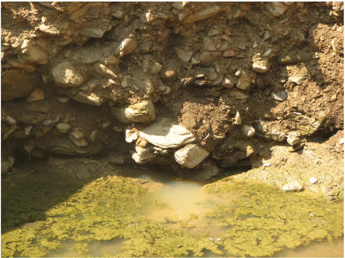
Plate 4.3 Unconsolidated gravel mixed silty material constituting the Valley-fill aquifer in the Mhadei River watershed
