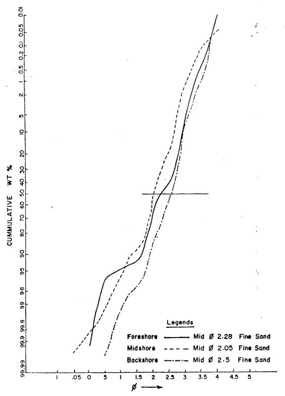
FIG. 11 SAND GRAIN SIZES : VARKA
