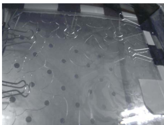
Figure 4. Photograph indicating cracked PADC sheets
