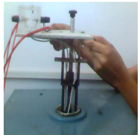
Fig7.1(b) D.C.Resistivity measurement Apparatus. Fig 7.1(c) Electrode assembly with sample
