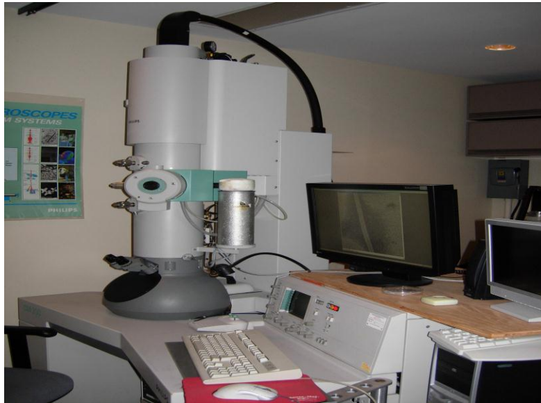
Fig. 5.2 (a) : TEM Philip model CM 200, electron beam of 200KeV
