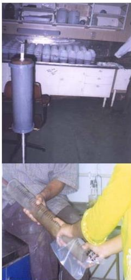
Fig. 2.2: Photograph of the two sediment sub-samplers (fixed and hand held) used on-board for sub sampling the cores, fixed one designed by Valsangkar (2007).
