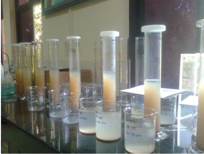
Fig. 2.3: Pipette analysis of the studied cores in progress
