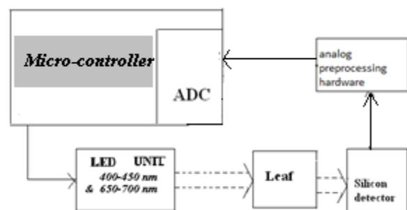
Fig 1: Block diagram of construction of the system
