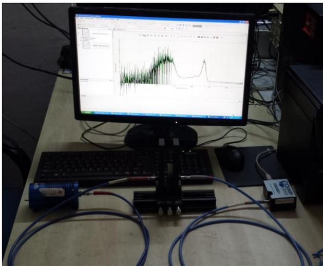
Fig 2: Picture of experimental setup; with Quartz Tungsten Halogen (*QTH*) Lamp (light source), cuvette holder and Spectrometer USB 2000+ (Left to right).
