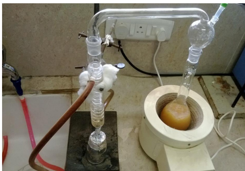
Figure 4.1: Distillation unit used for distillation of fermented cashew apple juice.
