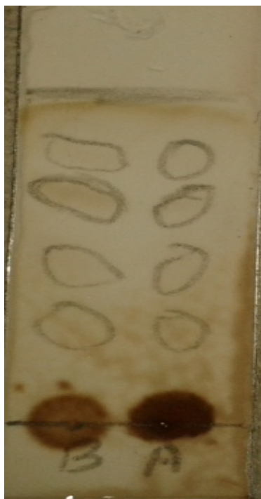
Fig. 7-e: Spots detected on TLC plate (A) aqueous fraction and (B) butanol fraction of methanol root extract of G. nervosa .
