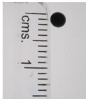
(B) Iron nanoparticle entrapped in Ca-Alginate bead
