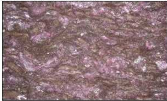
3. Stained slide of Stromatolitic Micrite. Calcitic micrite is pink stained, the white is silicious.
