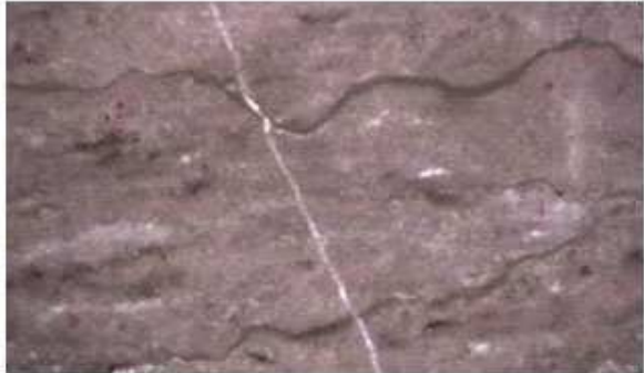
4. Laminated algal micrite showing stylolitic boundaries. Also seen in the section a quartz filled vein.
