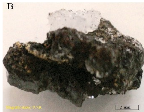
Figure 2. Basalt rock sample A) initial day and B) end day of experiment where crystal formation happen due to bacterial activity.
