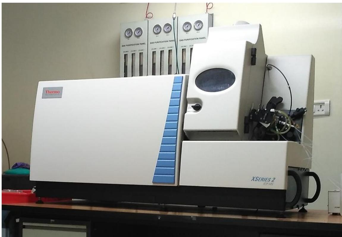
**Fig. 2.4:** *Inductively Coupled Plasma Mass Spectrometer (ICP-MS) facility at CSIR-National Institute of Oceanography, Goa.*
