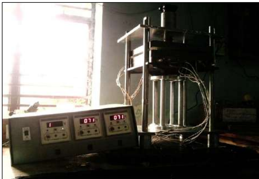
Figure 4.12: Modified polymer press with auxiliary heating controller
