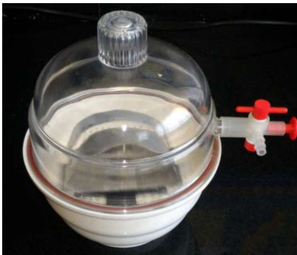
Figure 2.31: Exposure of polymeric film detector to ^{252}\text{Cf} source under vacuum for alpha sensitivity study.
