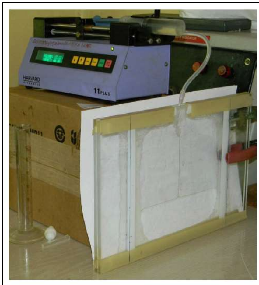
Figure 4.15: Filling a polymerization mould with syringe pump.
