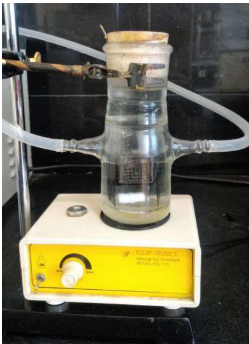
Figure 2.30: Glass assembly for chemical etching of polymeric detector.
