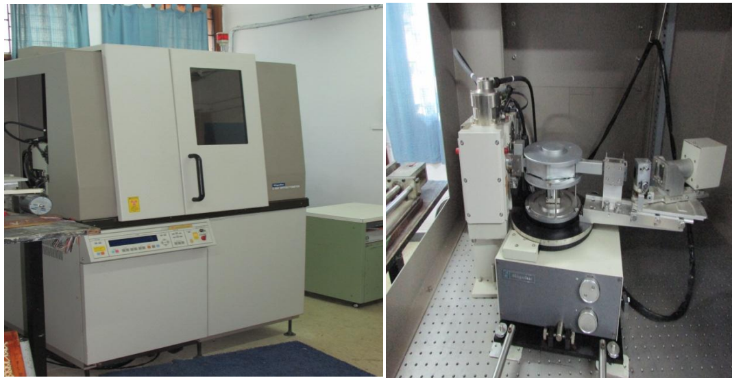
Figure 3.2.3 a) Rigaku X-Ray diffractometer, Department of Physics, Goa University, b) goniometer with Bragg Brentano geometry.
