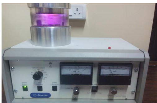
Figure 3.4.3 Process of gold sputtering using sputtering unit, Instrumentation centre, Goa University
