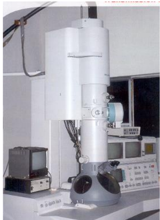
Figure 3.5.1 a) Basic construction of scanning electron microscope, b) PHILIPS CM200 transmission electron microscope at IIT Bombay, Mumbai-India
