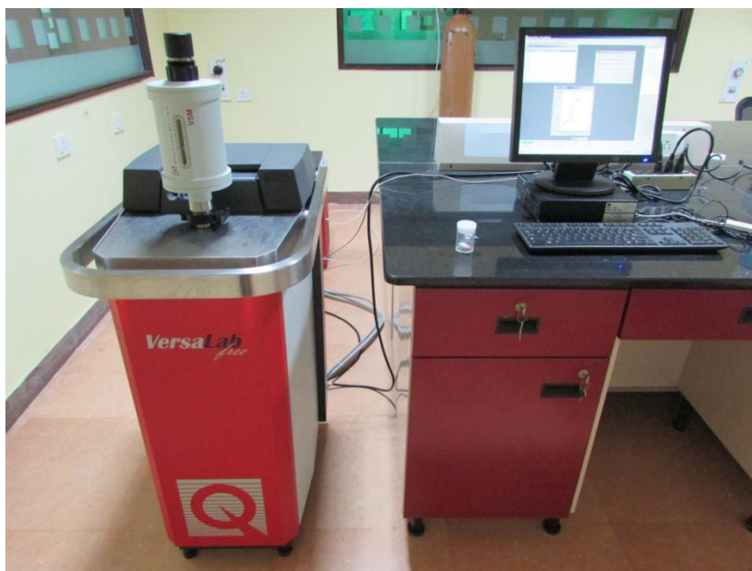
Figure 3.6.1 Quantum Design's Versa Lab 3 Tesla Vibrating sample magnetometer (VSM), Department of Chemistry, Goa University
