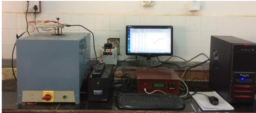
Figure 3.8.1 Two probe D.C. Resistivity setup with data acquisition system, Department of Physics, Goa University
