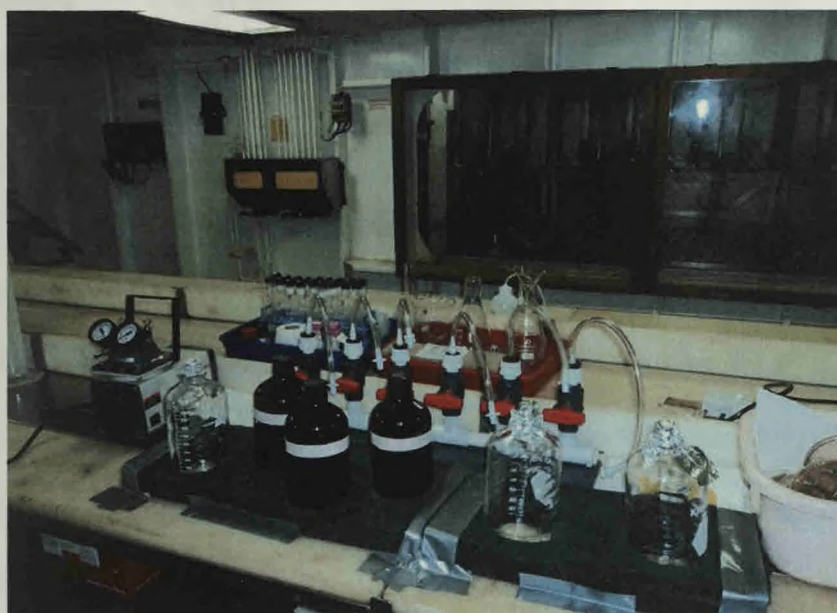
Plate 2.7 Filtration set-up for C-DOM analysis on board Sagar Sampada (Cruise SS286, Mar-2011).
