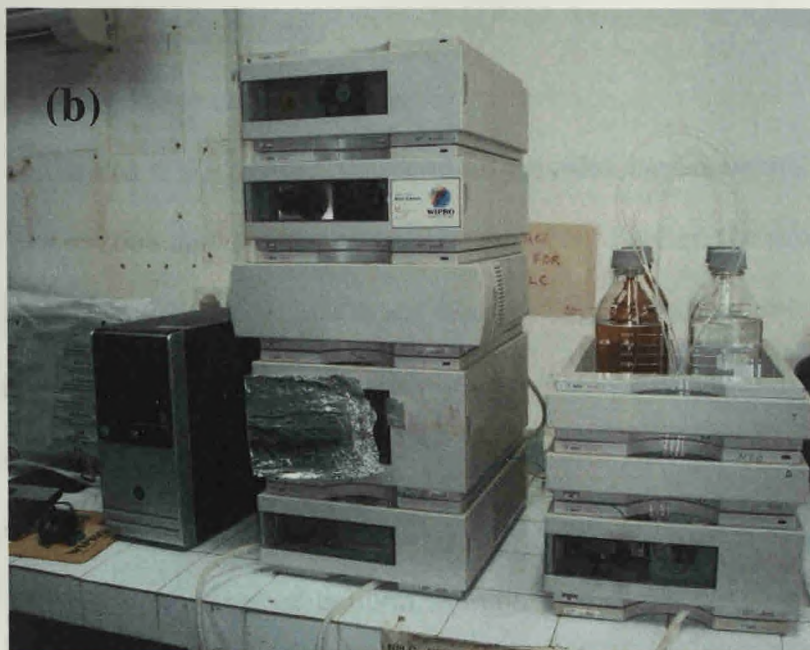
Plate 2.3 (a) Work space for filtration of water samples on board; and (b) Agilent 1100 HPLC facility used at National Institute of Oceanography (CSIR-India), Goa.
