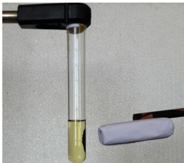
Fig. 17 – Fe-Ni-B nanocomposites showing magnetic behaviour
