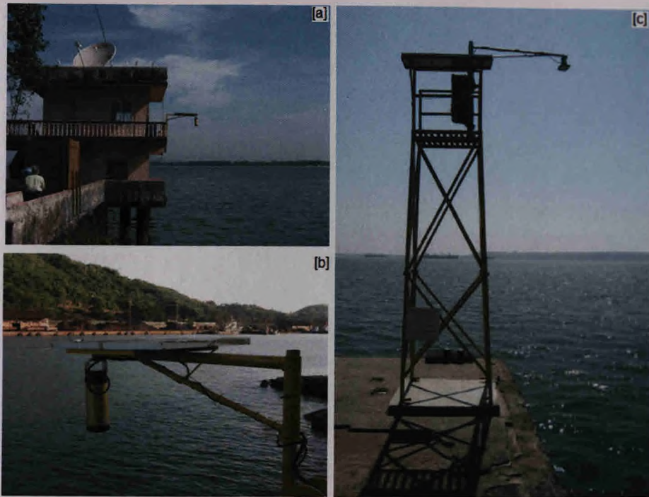
Figure 2.6. Typical installation of downward-looking aerial microwave radar sensor based sea-level gauges incorporated in the NIO's ICON at [a] Karwar, [b] Port Blair and [c] Dona Paula.
