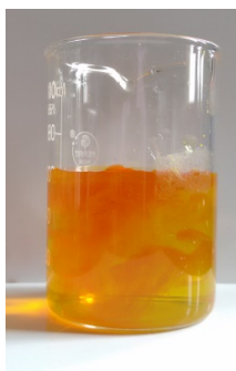
Fig. 1 Addition of ferric solution results in the formation of brown hydrous iron oxide. For a complete sequence of the crystal growth reaction see Fig. S1.
