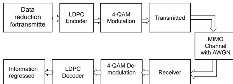
**Figure 1.**The proposed Sensor’s Data Transmission over 2,4,8-QAM Using LDPC Error Corrections Over MIMO Channel
