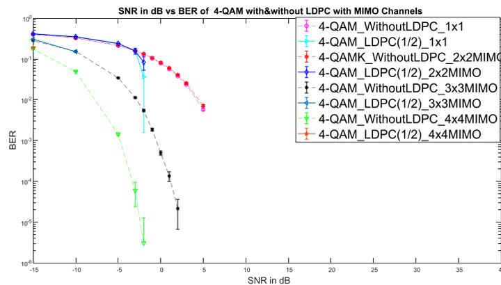
**Figure 3.** BER performance LDPC code with code rate  $R = 1/2$  over an AWGN channel via 4-QAM modulation.
