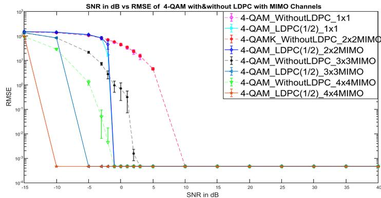
**Figure 2.** RMSE performance LDPC code with code rate  $R = 1/2$  over an AWGN channel via 4-QAM modulation.
