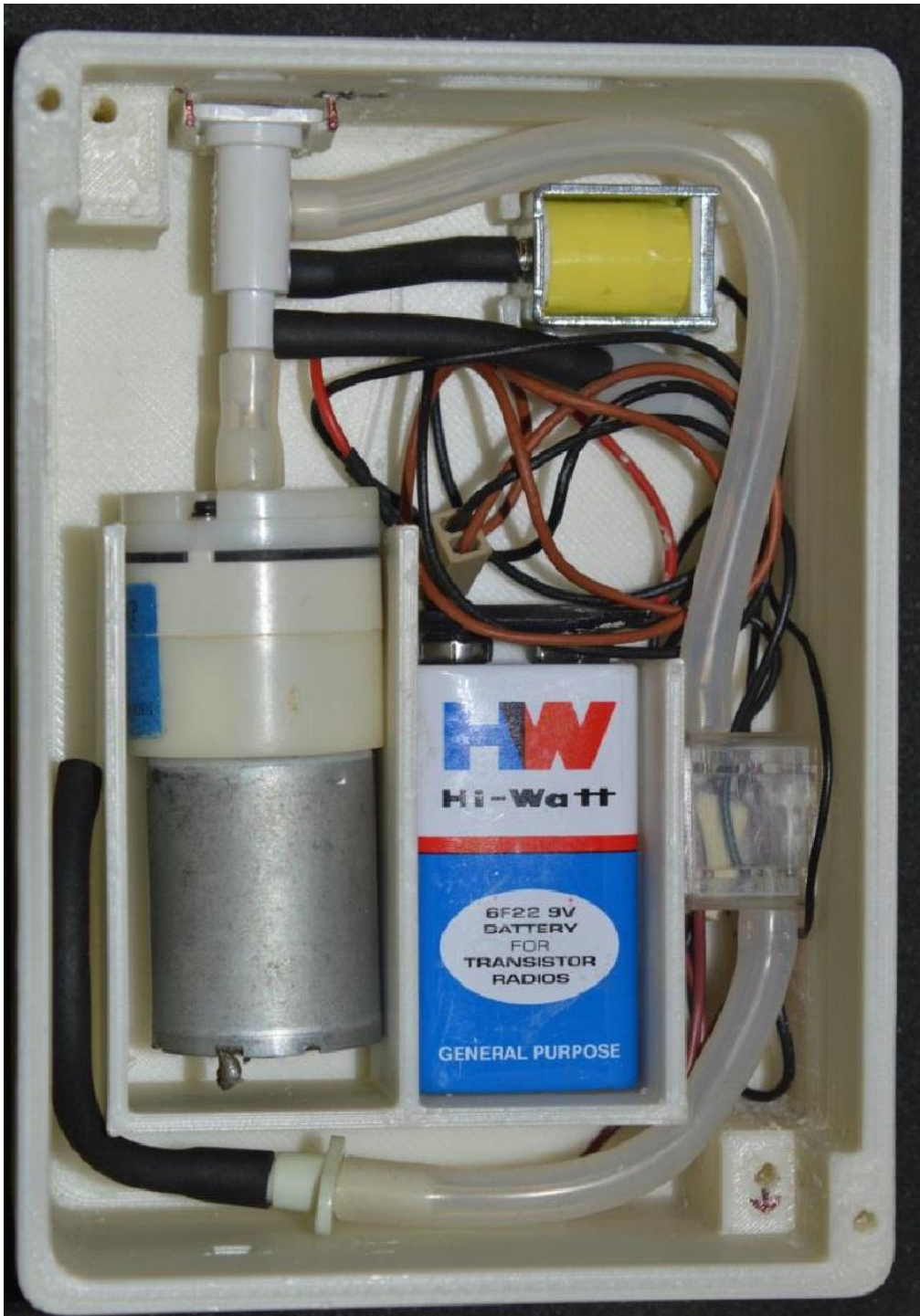
Figure3.14: The meter assembled in custom design box using 3-D printing for various components
