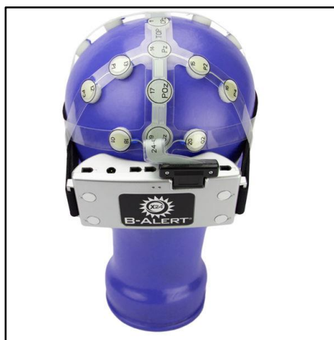
Figure6.7. B-Alert headset with 20 EEG sensor strip mounted on a scalp model
