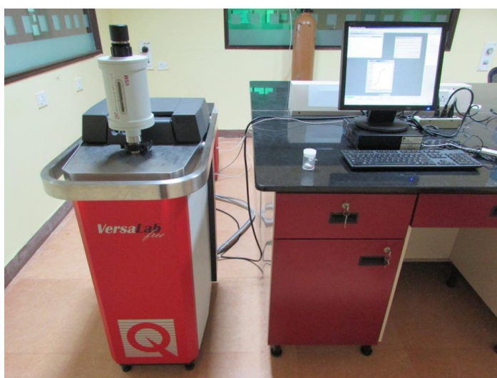
Fig. 2.11. Quantum Design's Versa Lab 3 Tesla Vibrating sample magnetometer (VSM), Department of Chemistry, Goa University.
