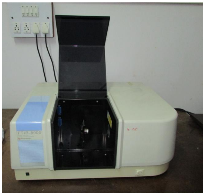
Fig. 2.5. Shimadzu FTIR 8900 assembly, Department of Physics, Goa University
