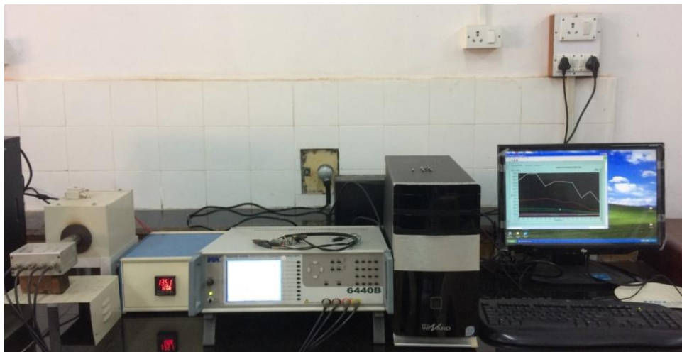
Fig. 2.12. WAYNE KERR 6440B Precision component analyzer, Department of Physics, Goa University, Goa.
