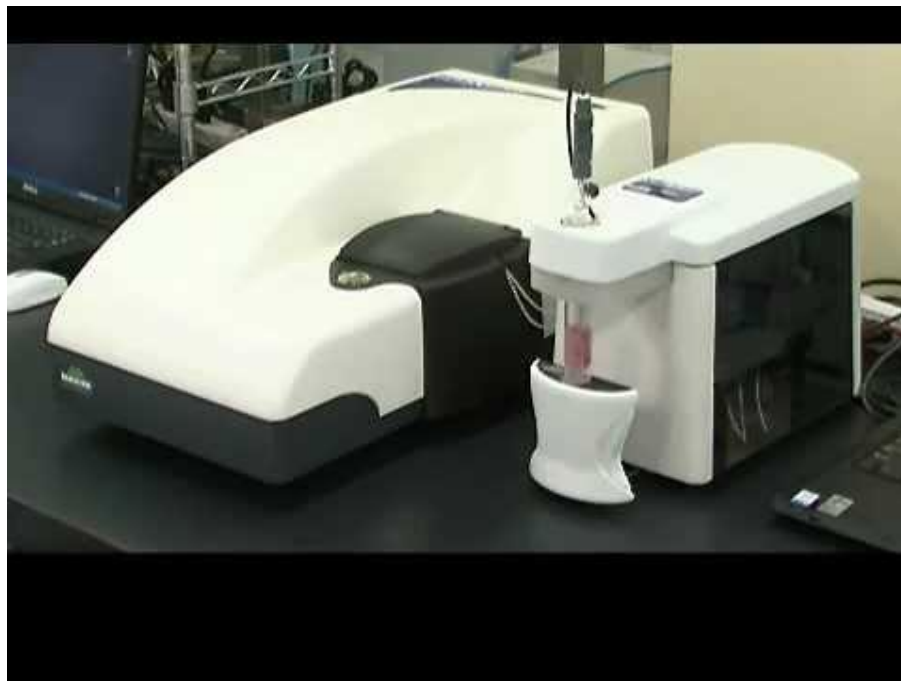
Fig. 2.4. Zetasizer Nano Malvern instrument, Materials Research center, MNIT, Jaipur.
