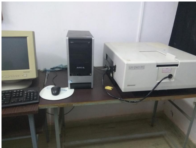
Fig. 2.6. SHIMADZU 2401 PC UV-Vis spectrophotometer, Department of Physics, Goa University.
