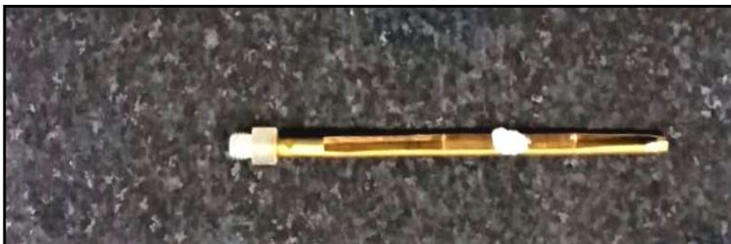
Figure 3.8.2: VSM sample holder and the sample wrapped in Teflon tape.
