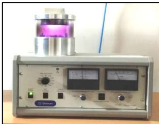
Figure 3.4.3: Sputtering process using sputtering unit.
