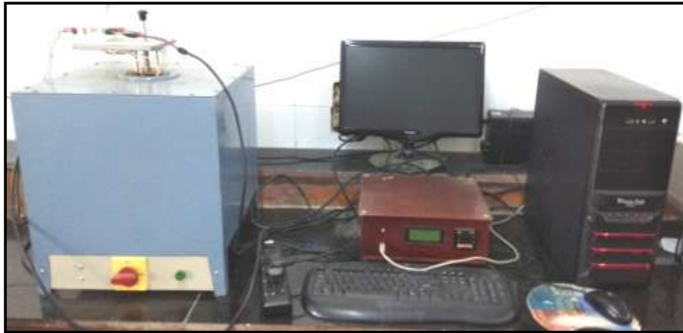
Figure 3.10.1: Two probe D.C. Resistivity setup with data acquisition system.
