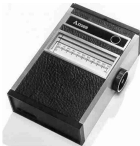
Figure 1.3: Ames Reflectance Meter
