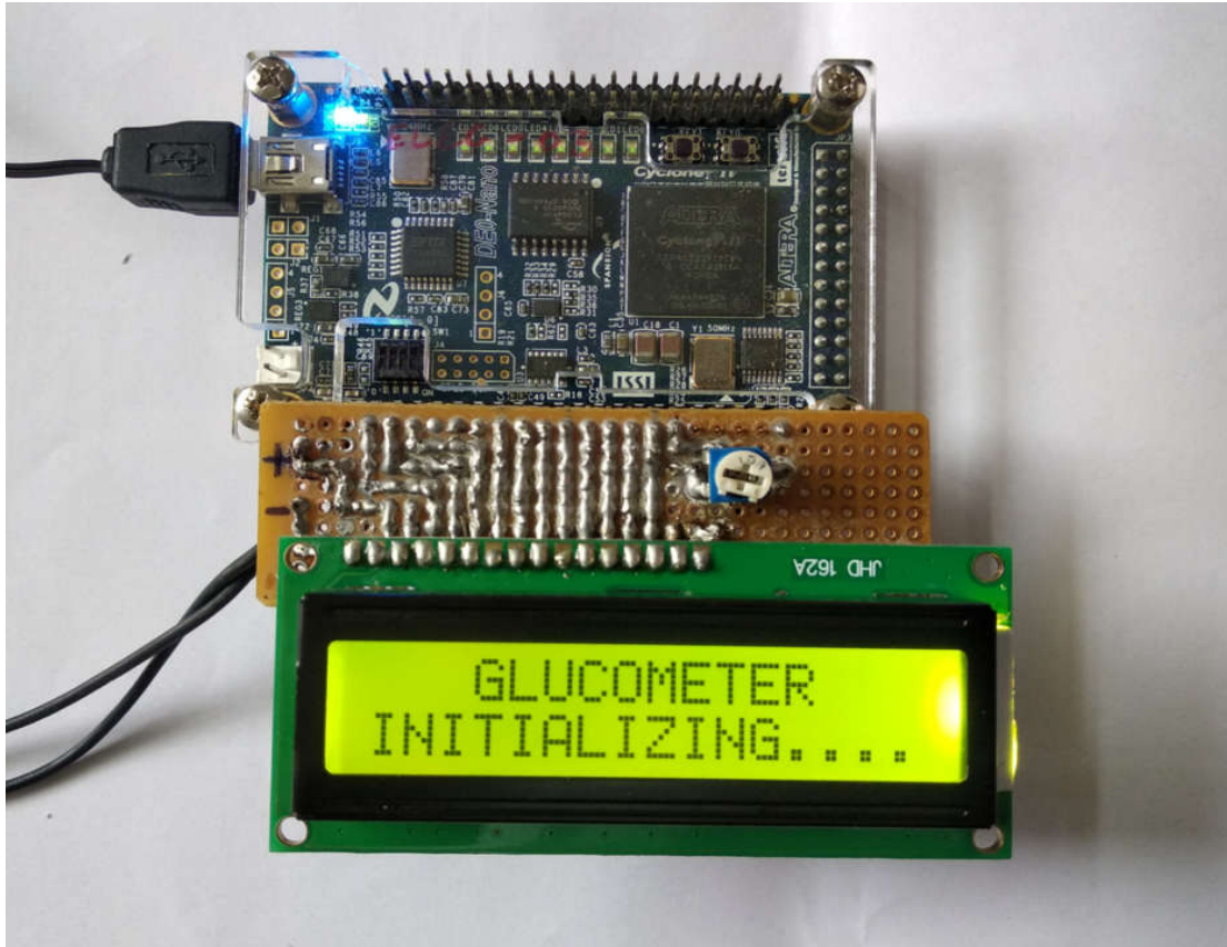
Figure 5.13: NIOS-II configured on DE-0 Nano board
