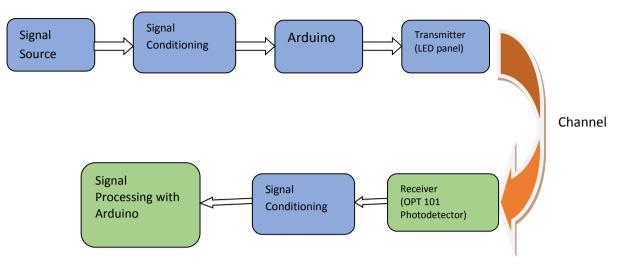
Fig. 2. System Implemented Block
