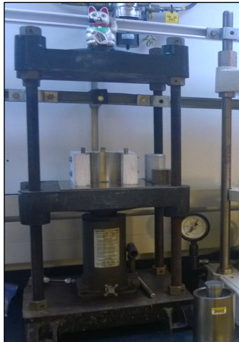
Fig 2.6. Titanium and Steel Squeezing Device Onboard JOIDES Resolution
