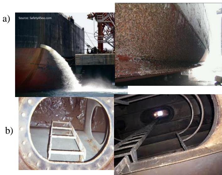
Figure 1.6 Images showing (a) clean and fouled surface of a vessel, (b) interior of an ocean-going ship's ballast tank (Sources: https://www.environmental-expert.com/products/harsonic-for-the-hull-of-vessels-674499 , https://www.usgs.gov/media/images/ballast-tank-ocean-going-ship ).
