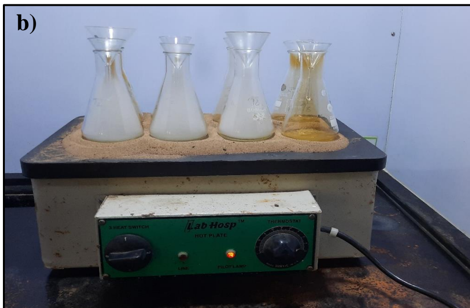
Plate 8.2: Sample digestion of Rhizophora mucronata plants: a. Reduction of acid content at high temperature; b. Appearance of white fumes after complete digestion of the sample.
