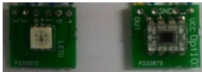
Figure 4.4: PCB fabricated with Multichip LEDs and OPT101.
