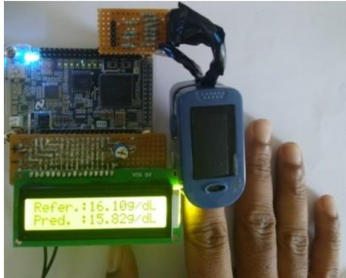
Figure 4.12: The designed haemoglobin measurement system.
