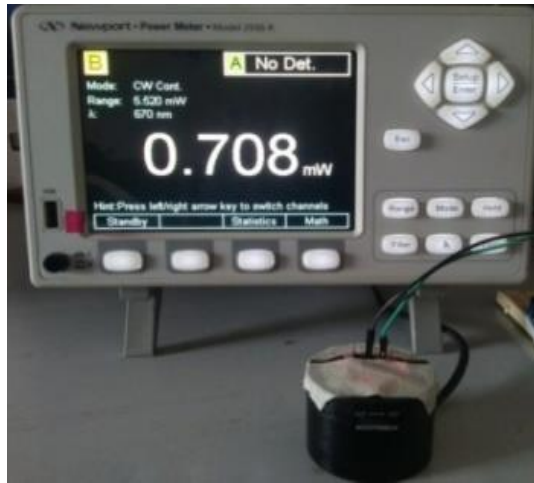
Figure 4.8: Standardization of LEDs power using Newport power meter.
