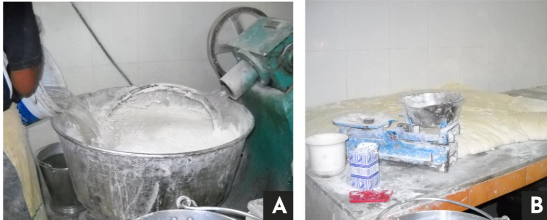
Fig. 4. A: Electric mixer; B: A small weighing scale to portion out the dough for individual loaves (Source: Authors)
