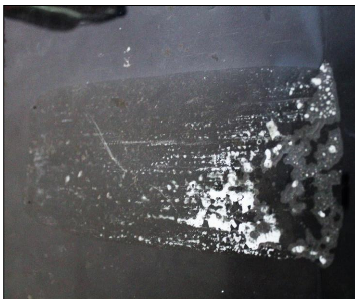
Figure 2.42 PSOC + CN (1:1 w/w; 2% TPP w/w) film on polyester support by film application technique
