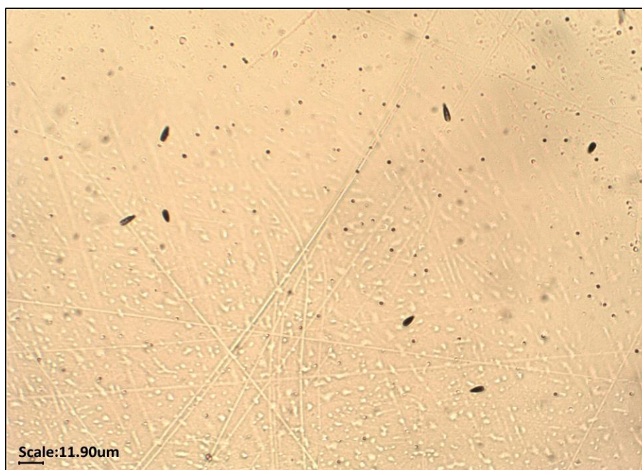
Figure 3.29 Fission fragments (black, 7-9 \mu\text{m} elongated trails) observed in poly (OESDAC-co-ADC; 1:1w/w) detector when etched for 1 minute in 3 N NaOH at 60°C (40x magnification).
