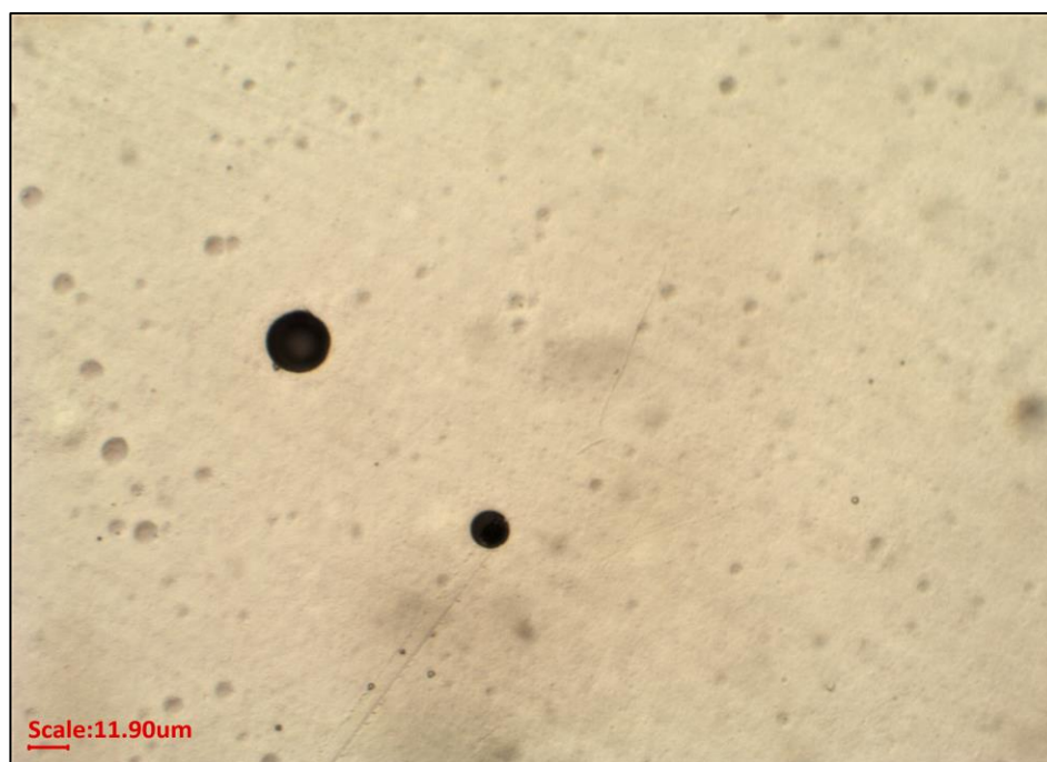
Figure 3.31 An alpha and fission tracks observed in poly (OESDAC-co-ADC; 1:1w/w) detector after 5 minutes of etching in 3 N NaOH at 60°C (magnification: 40X), pre-exposed to ^{252}\text{Cf} source at 3 cm height in vacuum for 24 hours.
