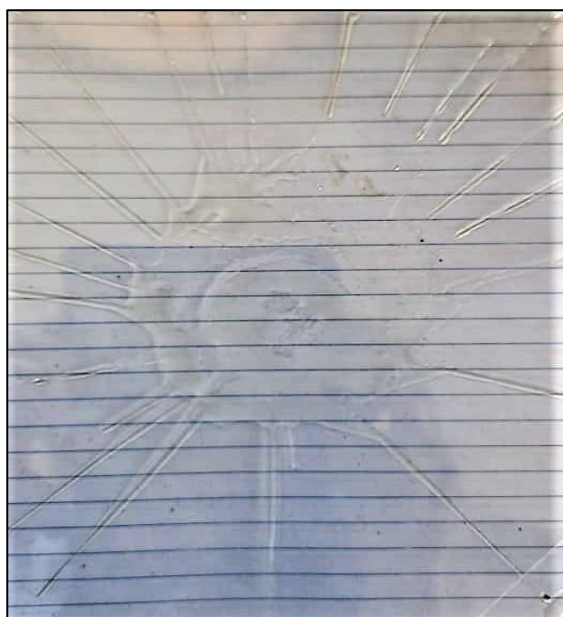
Figure 2.40 PSOC (100% w/v; 2% TPP w/w) film on polyester support by spin coating technique
