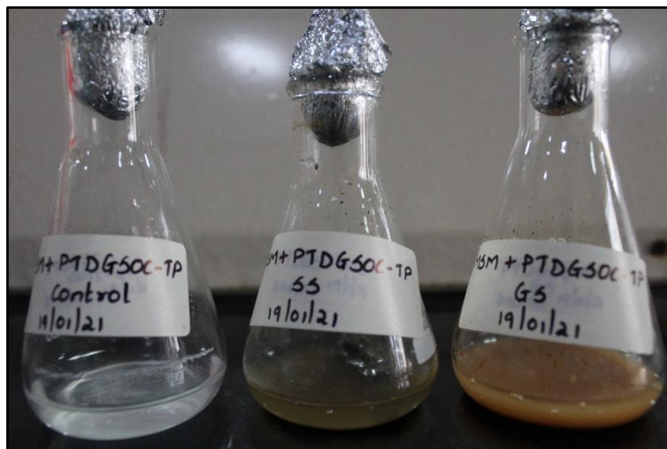
Figure 2.45 MSM broth culture flasks for isolation of microbial isolates for degradation of PSOC linear APC (control with MSM broth+1% PSOC polymer; MSM broth+1% PSOC polymer + 1% sewage sludge sample; MSM broth+1% PSOC polymer+ 1% garden soil sample).
