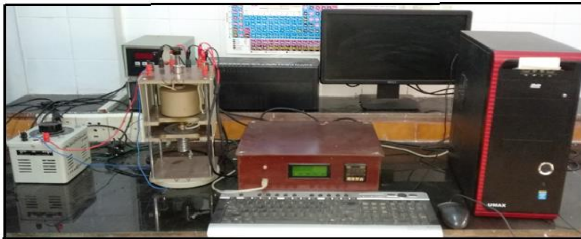
Figure 2.9: Thermopower setup, School of Physical and Applied Sciences, Goa University.
