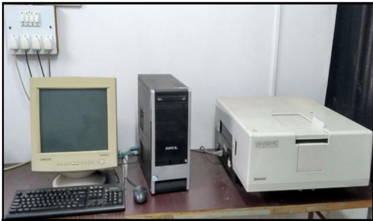
Figure 2.5(a): SHIMADZU 2401 PC UV-Vis Spectrophotometer, School of Physical and Applied Sciences, Goa University.
