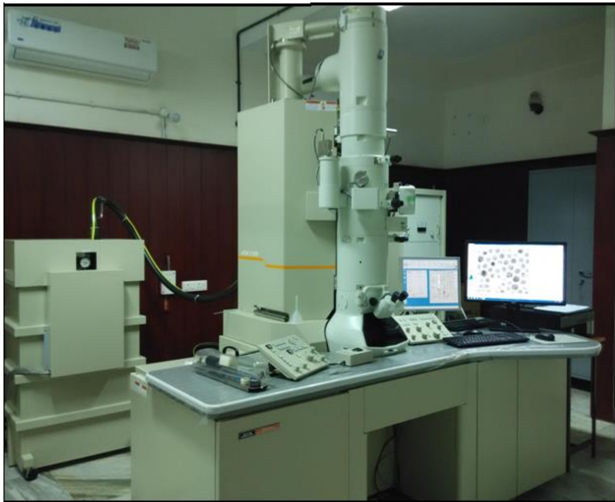
Figure 2.4(b): HRTEM JEOL/JEM-2100, with an accelerating voltage 200KV DST-SAIF, Kochi.
