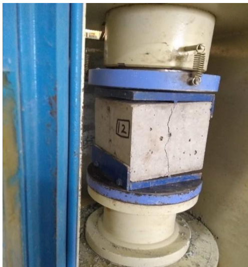
(c) splitting of specimen
