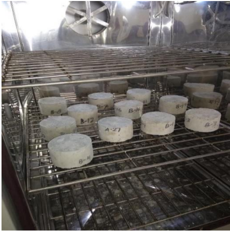
(a) test specimen ready for conditioning
