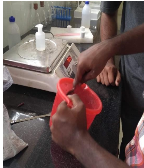
(b) Addition of water and mixing
