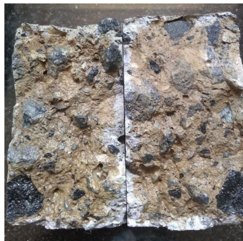
(g) depth of chloride penetration in specimens
