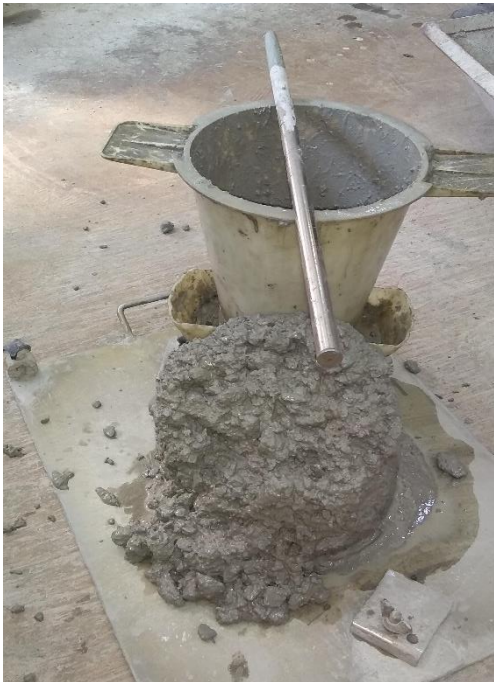
(c) removal of slump cone
