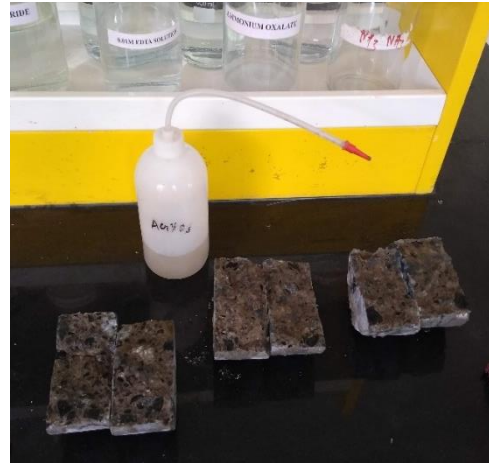
(f) spray of silver nitrate after splitting
