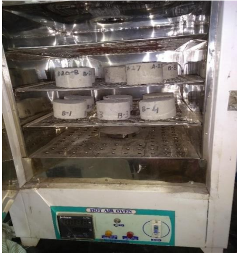
(a) Specimen ready for drying in oven
