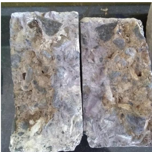
(g) depth of chloride penetration in specimens
