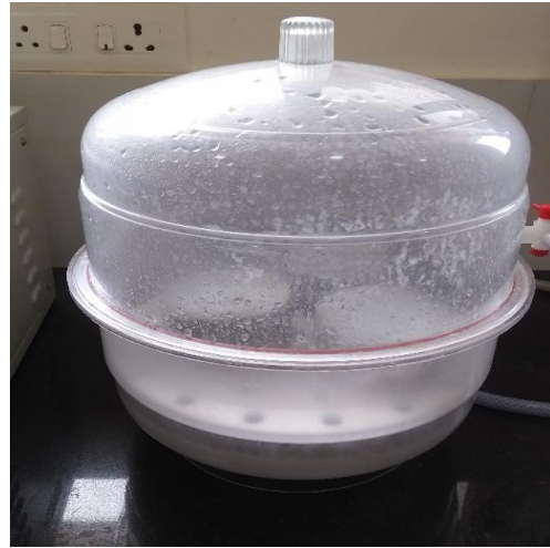
(b) preconditioning in vacuum container
