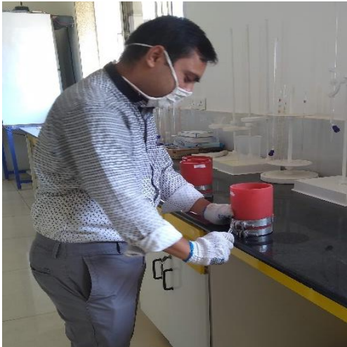
(c) fitting of rubber sleeve on specimen
