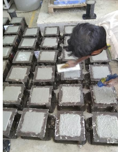
(b) Casting 150 mm cubes of concrete
