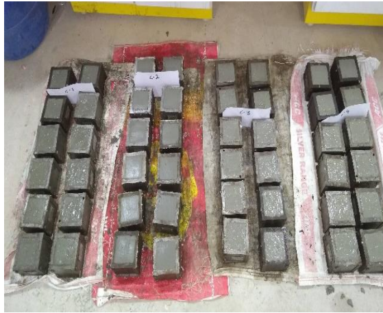
(a) Casting of 70.6 mm mortar cubes
