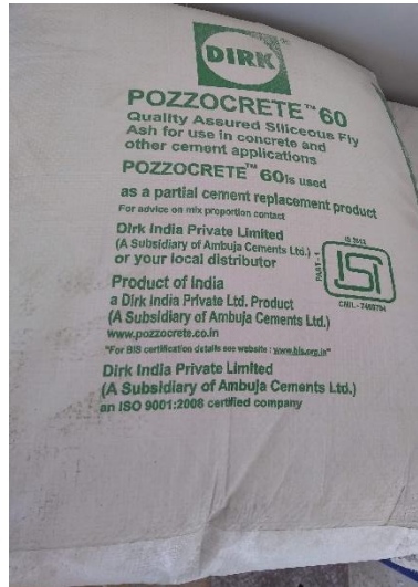
Figure 3.2. Fly ash (POZZOCRETE 60) used in the present study.
