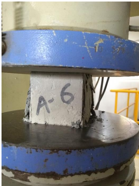
(c) Testing of mortar cube for compressive strength
