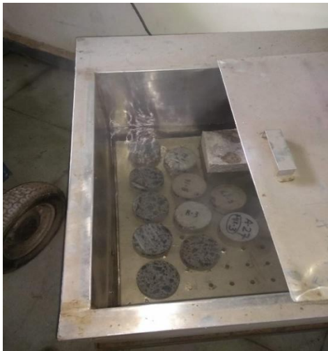
(c) saturated specimens under boiling condition
