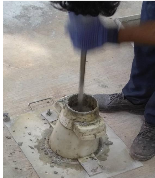
(b) tamping of concrete
