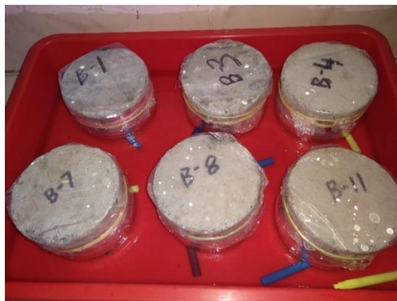
(e) placement of specimen for water absorption at different intervals
