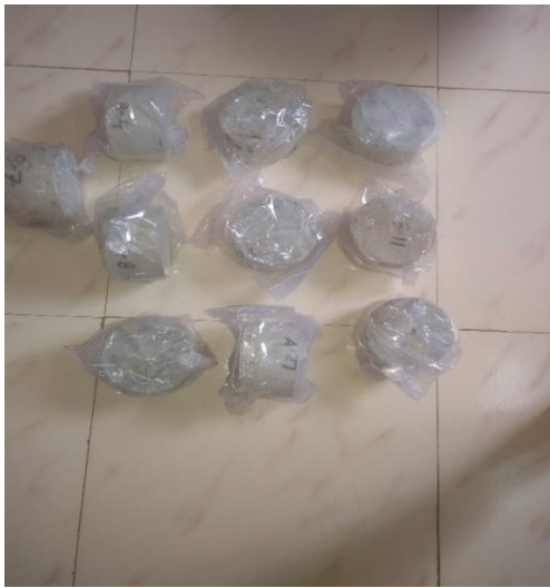
(c) specimen in sealable container
