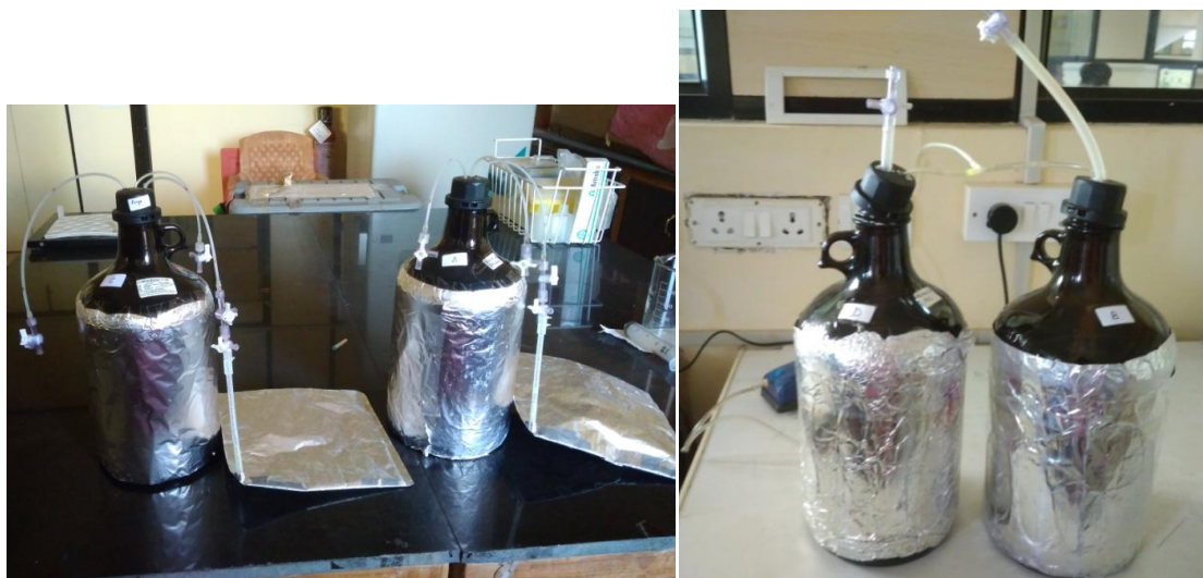
Figure 5.2: Experimental setup used in the laboratory, two bottles were oxygen-limited by purging of N_2 gas in the headspace (left), and two bottles were aerated using an aerator (right).
