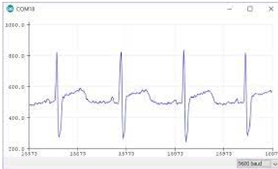
Figure 4.14: ECG information measured using AD8232
