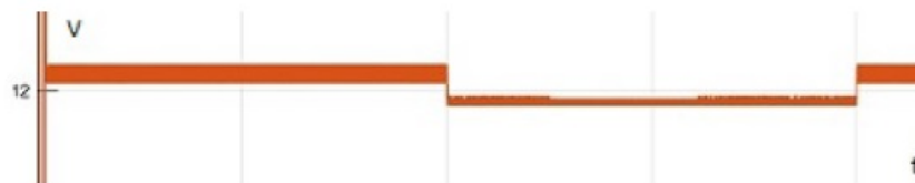
Figure 3.16: Buck Converter Output with Lead compensation model
