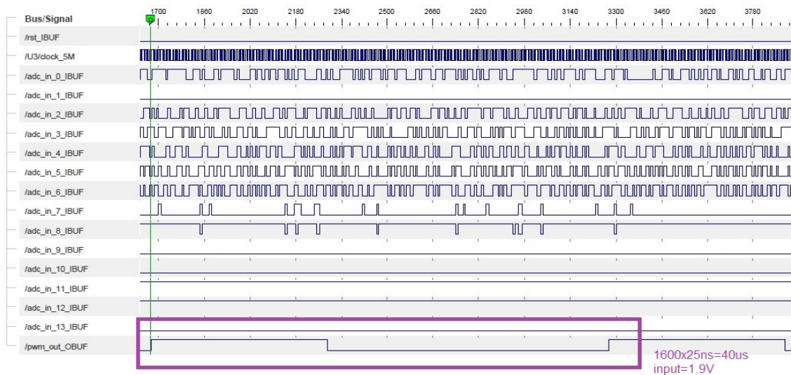
Figure 5.19: Real Time Simulation on Chipscope Logic analyzer for ADC input 1.9 V
