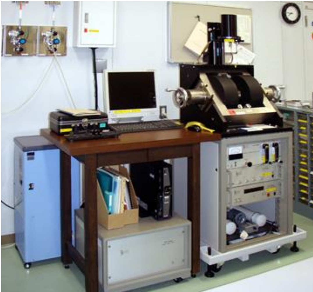
Figure 2.8: Vibrating Sample Magnetometer (VSM) housed at Paleo and Rock Magnetism Laboratory of CMCR, Kochi, Japan.
