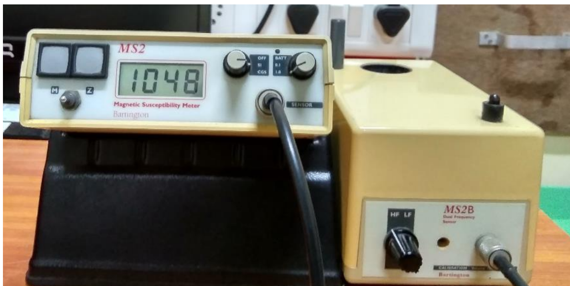
Figure 2.3: Bartington MS2B dual frequency magnetic susceptibility meter housed at Paleomagnetic laboratory CSIR-NIO, Goa, India.
