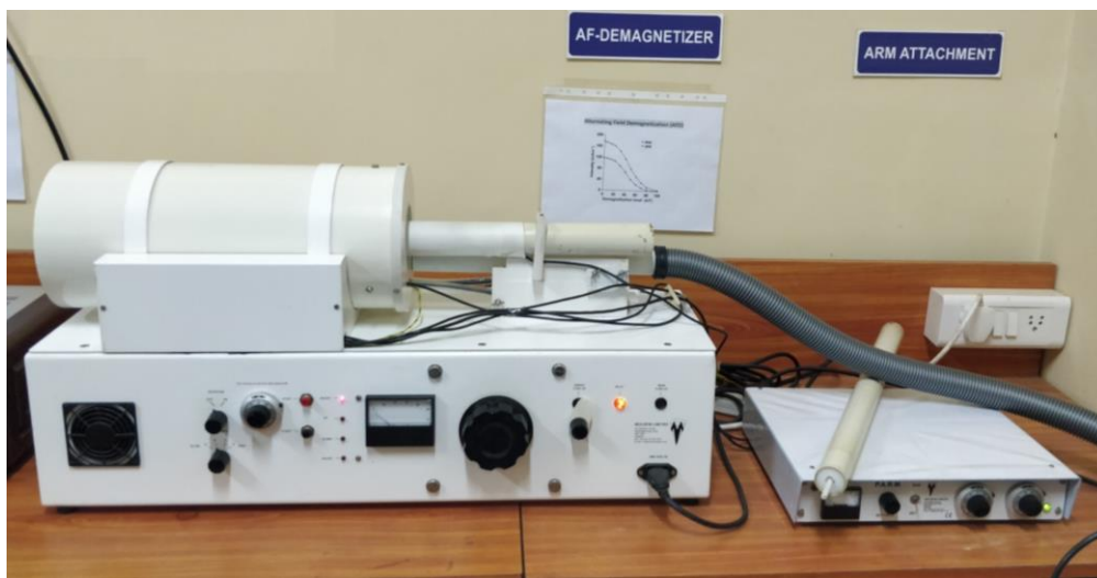
Figure 2.5: Molspin Alternating Field (AF)-Demagnetizer with p-ARM attachment housed at Paleomagnetic laboratory CSIR-NIO, Goa, India.
