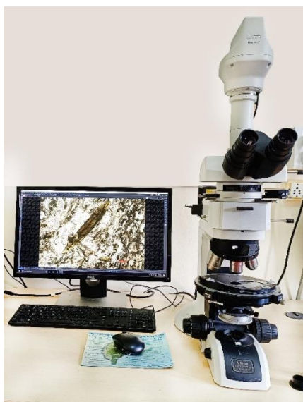
Figure 2.14: Petrographic trinocular microscope (Model No.-BX51TRF) housed at the Petrology Laboratory of CSIR-NIO, Goa, India.
