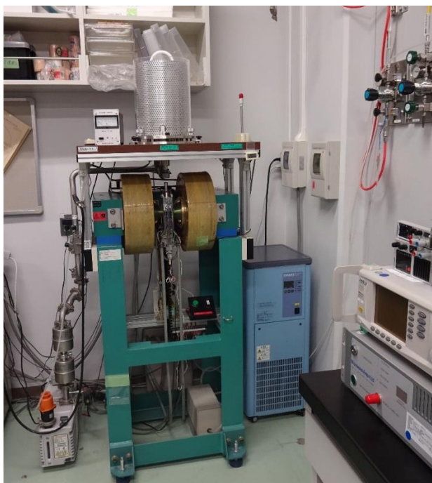
Figure 2.7: Natsuhara Giken (Model NMB-89) magnetic balance housed at Paleo and Rock Magnetism Laboratory of CMCR, Kochi, Japan.
