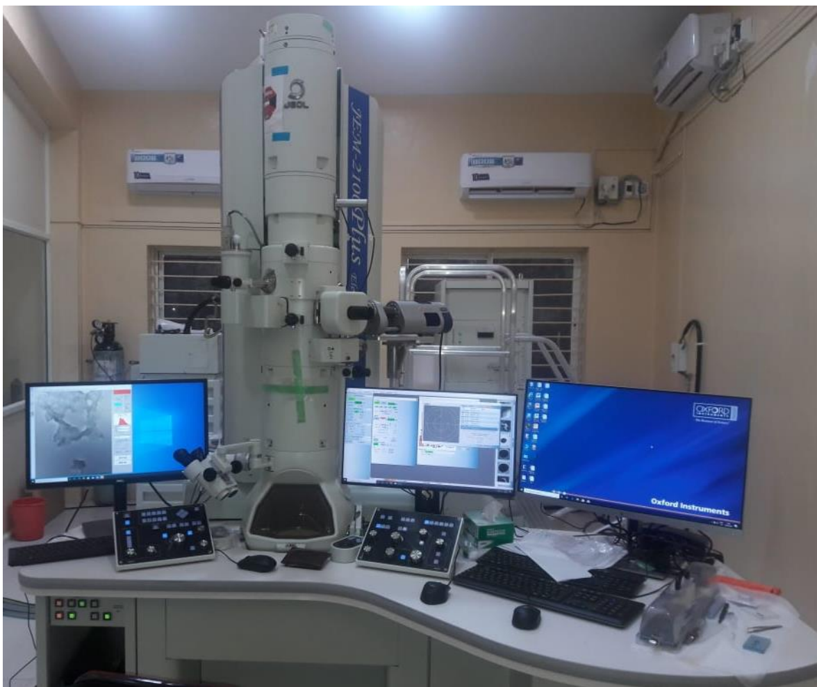
Figure 2.12: JEOL JEM-2100 Plus Transmission Electron Microscope (TEM) housed at Sophisticated Analytical Instrument Facility (SAIF), Shivaji University, Kolhapur, Maharashtra, India.
