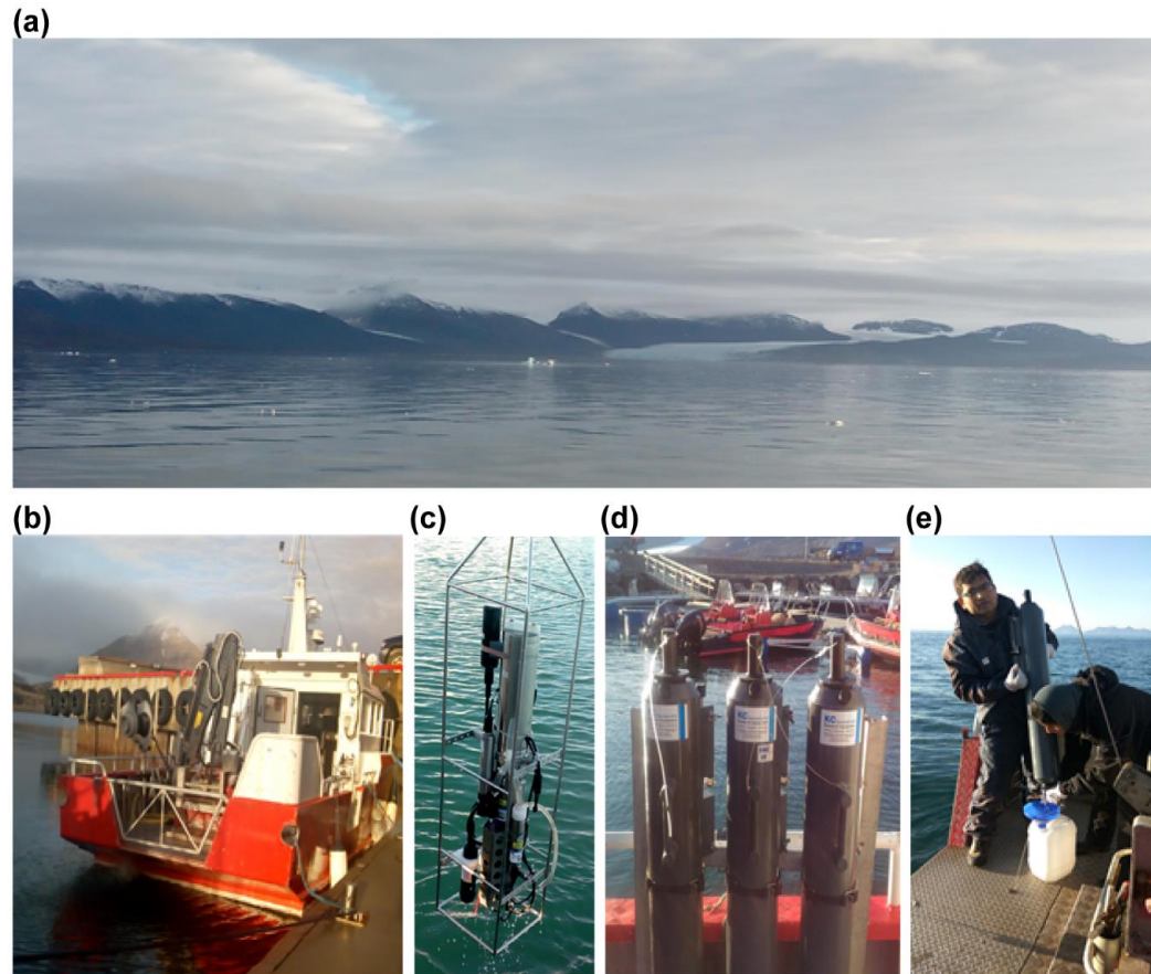
Fig. 3.3. (a) Kongsfjorden, (b) MS Teisten , the research vessel used for fjord sampling, (c) CTD operating from the vessel, (d) Niskin water samplers used for water sample collection, (e) Water sampling from the research vessel MS Teisten .
