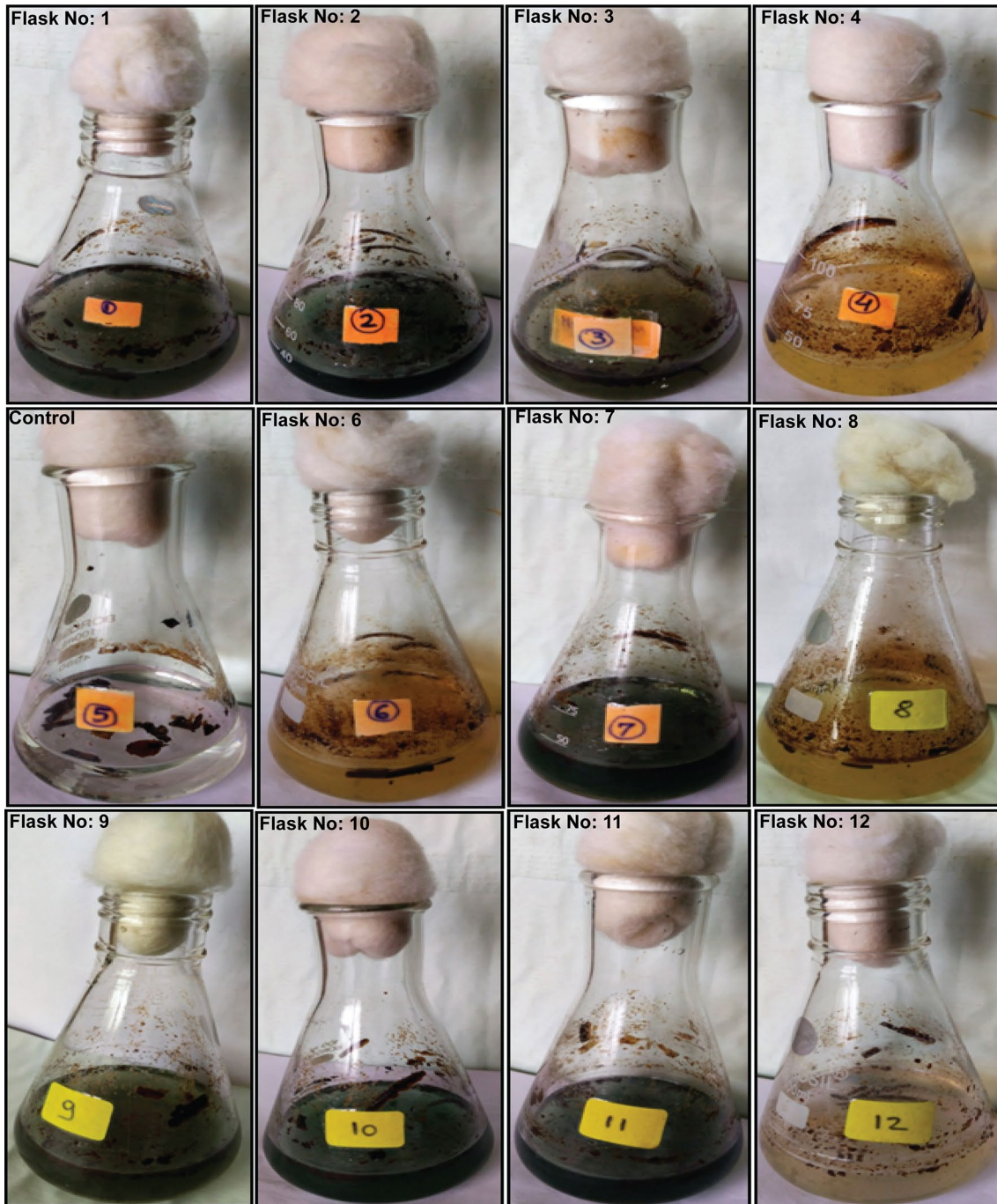
Fig. 1 Bacterial consortia used for studying the degradation of tarballs in the laboratory
