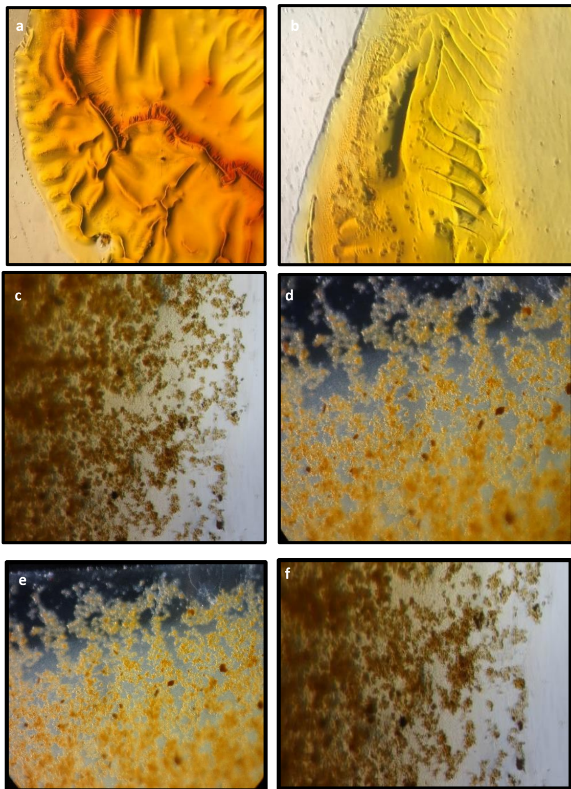
Figure 3.67(a-f): a,b-Film of Gold formed after dissolving in aquaregia indicating the formation of Gold; (c-f)- Gold formed at all the edges of the slide
