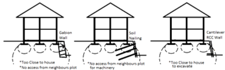
Figure A15.34 pressure bulb of the structure on the retaining wall and the different options explored by the owner
