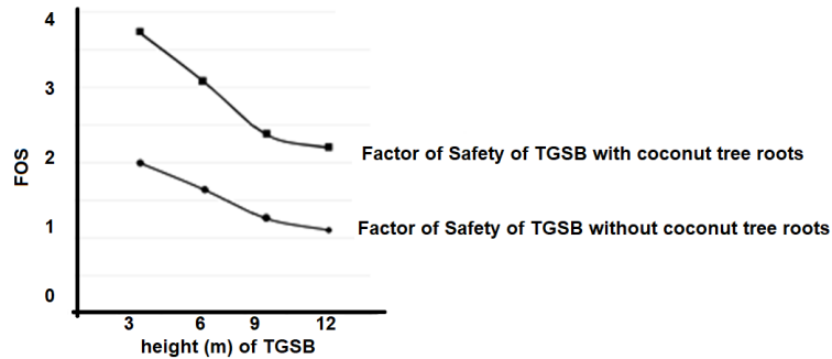
Figure. 5.10 Factor of safety for pseudo-static approach as per IS code
