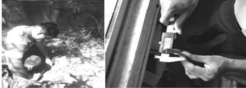
Figure 3.28 Measuring Coconut Tree Root Branching and Diameter using Digital Vernier Calliper
