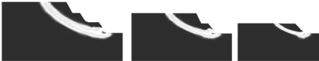
Figure 4.55 Stresses due to static forces in Midas analysis for 9m, 6m and 3m TGSB
