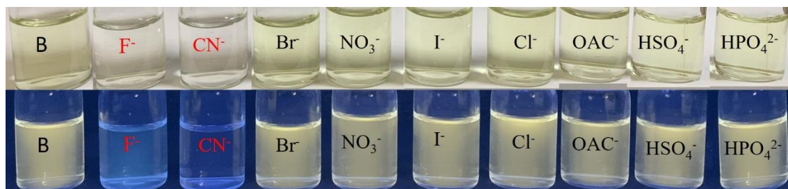
Figure 5.5. Photograph exhibiting fluorescence color change with addition of Fluoride anion in presence over other anions such as ( F^- , Cl^- , NO_3^- , Br^- , I^- , HSO_4^- , HPO_4^{2-} , OAc^- , CN^- ) in solution containing receptor 1 1-(p-tolyl)-4,9-dihydro-3Hpyrido[3,4-b]indole.
