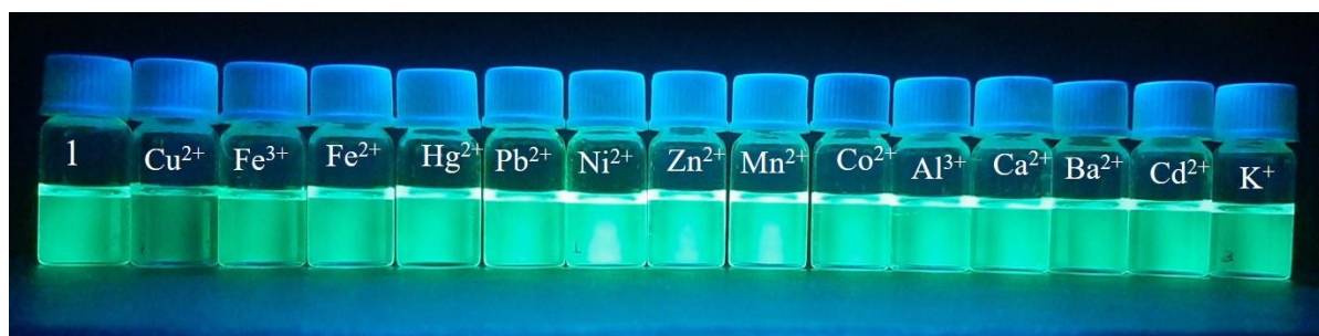
Figure 3.9. The sensing performance for DTBPA 1 over different cations representing the quenching of fluorescence upon addition of \text{Cu}^{2+} ion.
