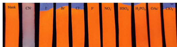
Fig. 11 Paper strip based selective detection of CN - ions with probe NDI-1, over other anions by the naked eye under 365 nm UV light.
