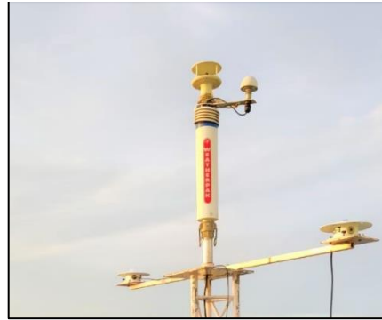
Figure 2.6 On-board installed Automatic Weather Station (WeatherPak®-2000 v3).
