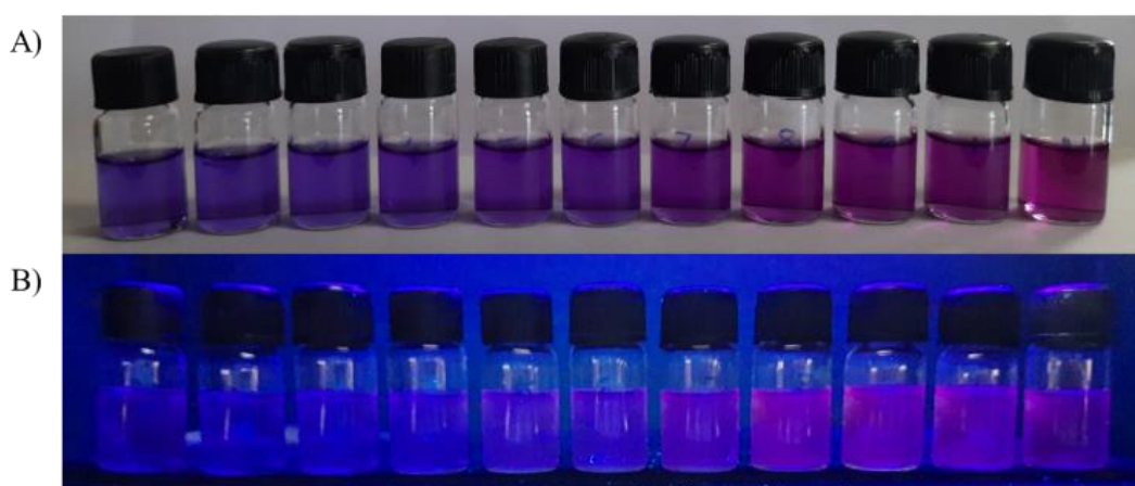
Figure 4: Sensing performance of the probe DDPT 1 (90 \mu M) in THF with the addition of trifluoroacetic acid (0.2 to 2 equiv) A) under visible light B) under UV light illumination at 365nm.
