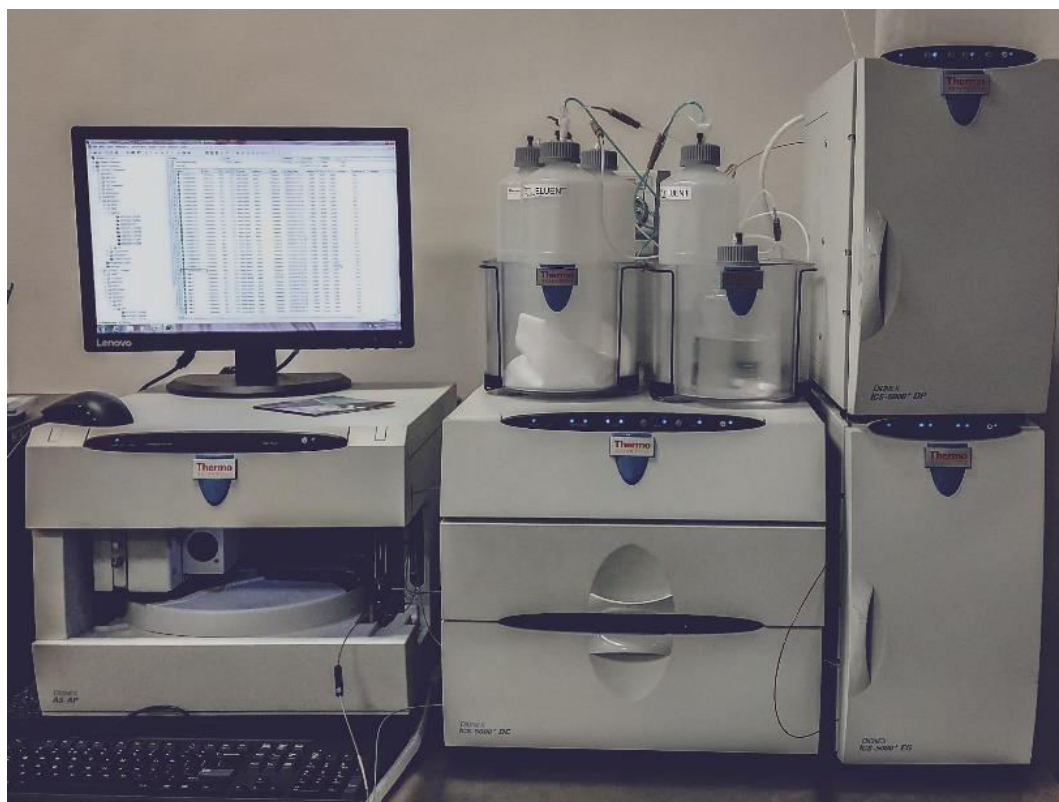
Figure 2.7. Ion Chromatograph (IC) instrument for cation and anion analysis housed in a Class-100 clean room at NCPOR, Goa.
