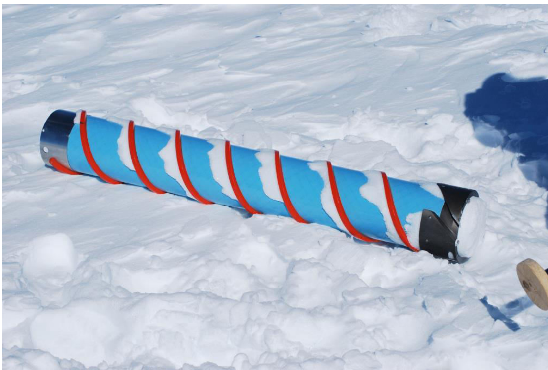
Figure 2.3. Drilling of snow cores was performed with a Kovacs Mark IV device with a 14 cm barrel diameter and snow cutters.
