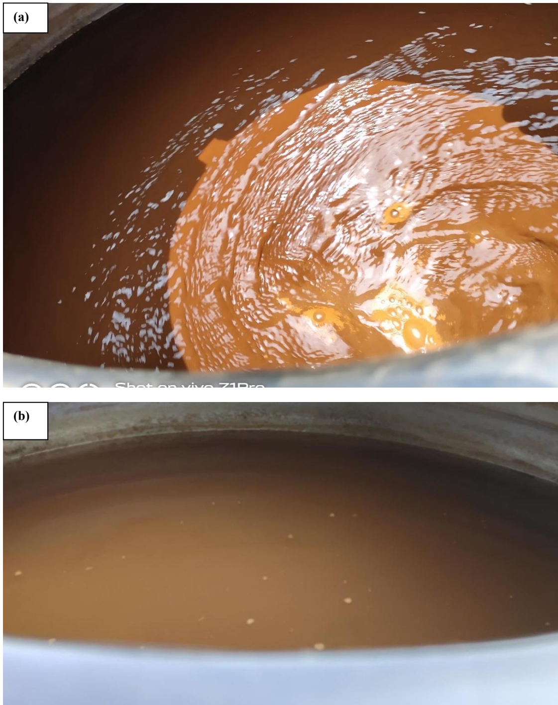
Figure. 3.48: Visible turbidity in control tank, (a) after 0 min of stirring (b) after 1 hrs of stirring In the 1000L of tank.
